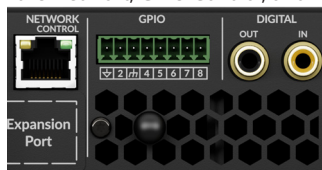
Ethernet Port, GPIO Control, and Digital Audio Input/Output
